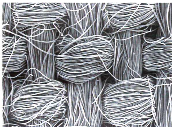
Flexzorb 100% Activated Carbon Cloth in Woven Form. Magnification x40
