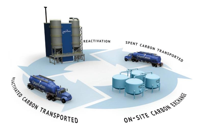
Calgon Carbon reactivation services include the reactivation of spent granular activated carbon on a pool or custom basis.
